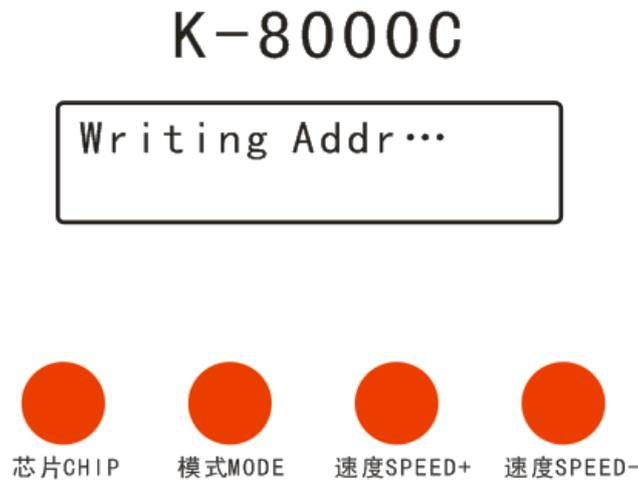
3. After finished address code, press “CHIP” first and at the same time press “MODE” button, switch to playback mode, switch the chip to Chip: 10, this is the DMX512 standard agreement 250K playback mode. At this time, press MODE button and SPEED button can separately switch playback mode and adjust speed, as below:
