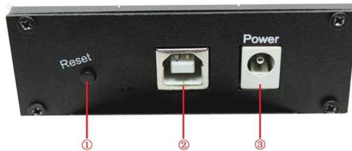
①It is the reset button, when the controller crash, can touch this key to reset.
