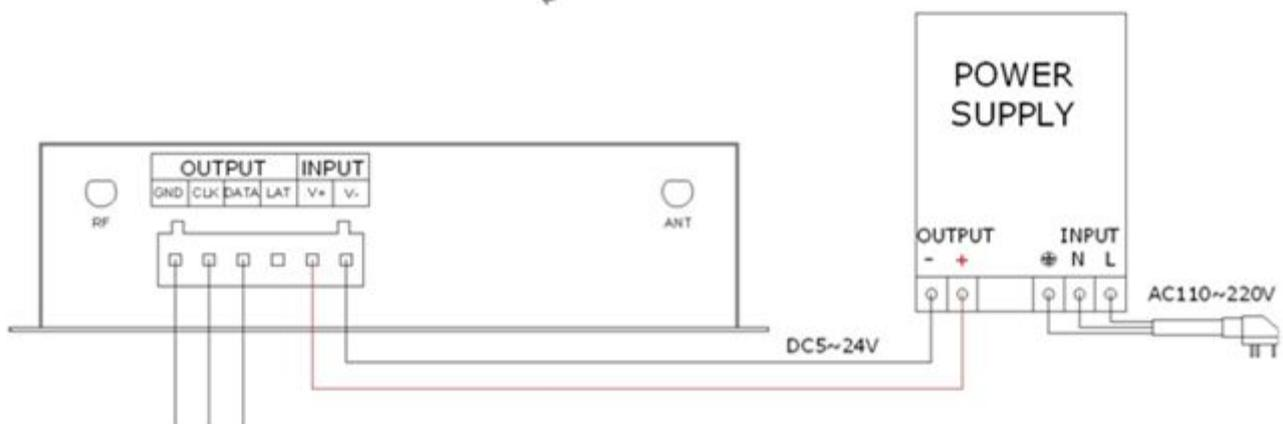
In above picture, if there are 2 signal lines, then you need to connect the ground wire, clockline, data line with GNG、CLK、DATA; if it is 1 signal line, then just need to connect the ground wire, data line with GND、DATA.
