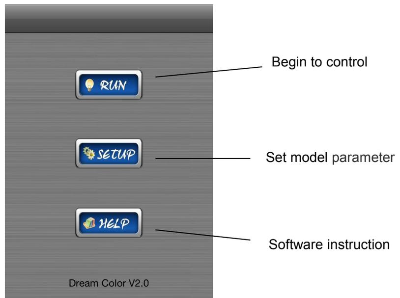
Above picture "RUN" is enter remote control interface, before enter this interface, need to set the software parameter first. Click the "SETUP" in middle to setting.
